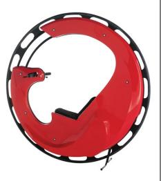
four-stroke engine, the Motorized Monocycle can transport you around town illegally at speeds of up to 25 mph. Steering is performed by leaning to one side, with brakes available ri ght on the handlebar. It features cushioned seats, padded footrests and a fiberglass body for durable performance. The giant-wheeled vehicle can handle riders up to 6'3" tall, provid-
